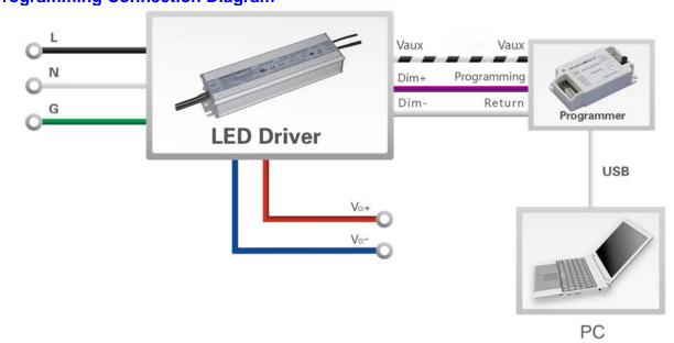
Note: The driver does not need to be powered on during the programming process.
