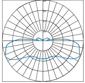
Maximum Candela = 834.97 Located At Horizontal Angle = 225, Vertical Angle = 68 # 1 - Vertical Plane Through Horizontal Angles (225 - 45) (Through Max. Cd.)
