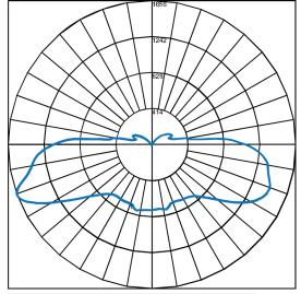
Maximum Candela = 1655.9 Located At Horizontal Angle = 135, Vertical Angle = 69 #1 - Vertical Plane Through Horizontal Angles (135 - 315) (Through Max. Cd.)
