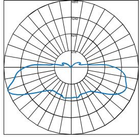
Maximum Candela = 1655.9 Located At Horizontal Angle = 135, Vertical Angle = 69 # 1 - Vertical Plane Through Horizontal Angles (135 - 315) (Through Max. Cd.)
