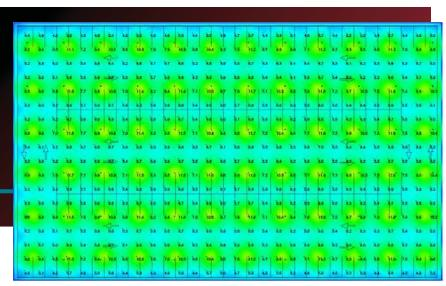
Computer Generated Rendering Fixtures mounted at 10' Quantity: 72 Wattage: 40W (CP40160) Fixture Lumens: 5,450 Average footcandle: 6.90FC Max. footcandle: 12.0FC
