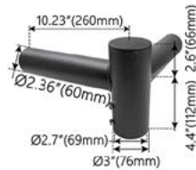
Description: Twin Spoke Accessory with 90° Arms Order Code: SP2H906BZ Color: Bronze Weight: 8 lbs.
