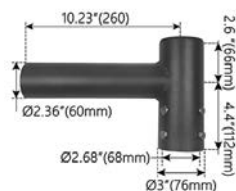
Description: Single Spoke Arm Order Code: SP1H6BZ Color: Bronze Weight: 5 lbs.
