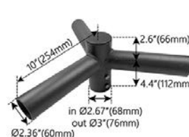
Description: Triple Spoke Accessory with 120° Arms Order Code: SP3H1206BZ Color: Bronze Weight: 10 lbs.
