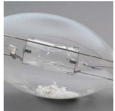
Ruptured arc tube contained within the intact outer jacket of a Venture MP lamp
