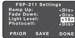
Displays the light level at the FSP-211. The light level reading can be used as a reference for setpoint adjustments.
