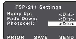
When the light level exceeds this setting, the lights will turn off even when the space is occupied. Once the light level exceeds this setting, the sensor will wait and monitor for a short period of time
