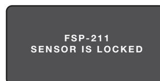
This screen will appear if the FSP-211 is locked. If it is locked, cycle the power.
