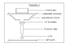
Strip Luminaire – Select a convenient location on the fixture where the LCTS will be visible after installation. Allow for proper clearance inside the fixture and drill or punch a 1/2" hole. Push the LCTS housing into the 1/2" hole and secure with nut. Connect the wires from the FHSCP-UNV to the LCTS (Violet to Violet, Brown to Brown). (Refer to Figure 4)
