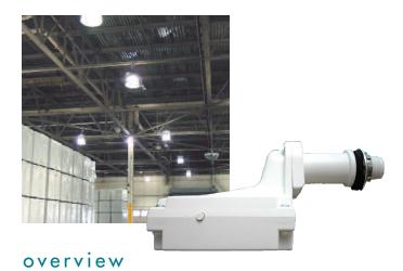
Venture Lighting's outdoor, wet-rated motion sensor utilizes Passive Infared (PIR) detection technology into a line voltage motion sensor. Designed to mount directly through a 1/2" knockout (7/8" hole) in a light fixture or pole, the sensor utilizes 100% Digital Passive Infared (PIR) technology that is tuned for walking size motion while preventing false tripping from the environment.
