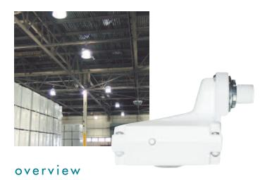
Venture Lighting's outdoor, wet-rated motion sensor utilizes Passive Infrared (PIR) detection technology into a line voltage motion sensor. Designed to mount directly through a 1/2" knockout (7/8" hole) in a light fixture or pole, the sensor utilizes 100% Digital Passive Infrared (PIR) technology that is tuned for walking size motion while preventing false tripping from the environment.
