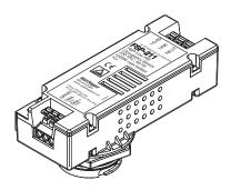
The FSP-211 is a motion sensor that dims lighting from high to low based on movement. This slim, low-profile sensor is designed for installation inside the bottom of a light fixture body. The PIR lens module connects to the FSP-211 through a 1.30" diameter hole in the bottom of the fixture.
