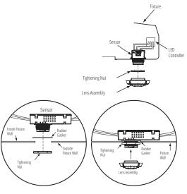
The Sensor accommodates fixture wall thickness up to 0.125" (3.18mm).
