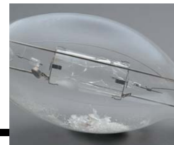
Ruptured arc tube contained in the intact outer jacket of a Venture MP lamp
