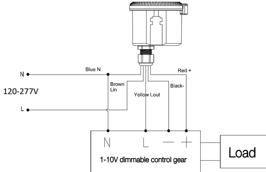
Figure 5: Wiring Diagram
