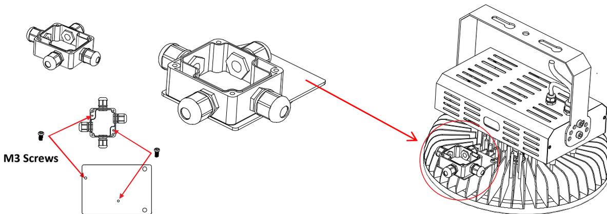
**STEP 3:** Attach sensor to fixture or reflector.
