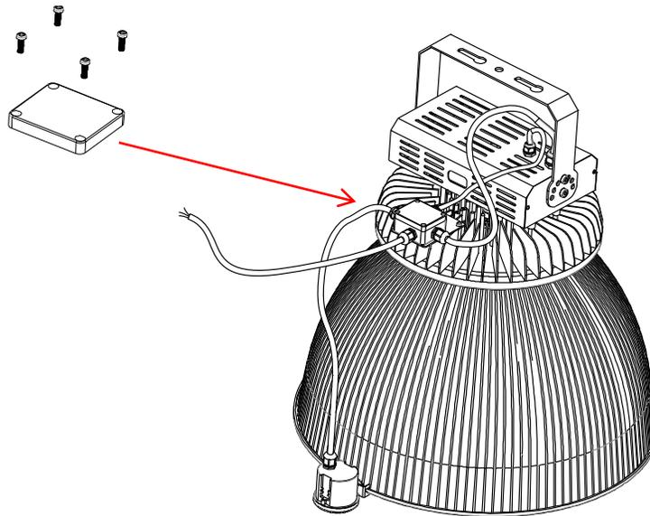
Figure 6: Attach cover to terminal block (fixture shown with reflector)
