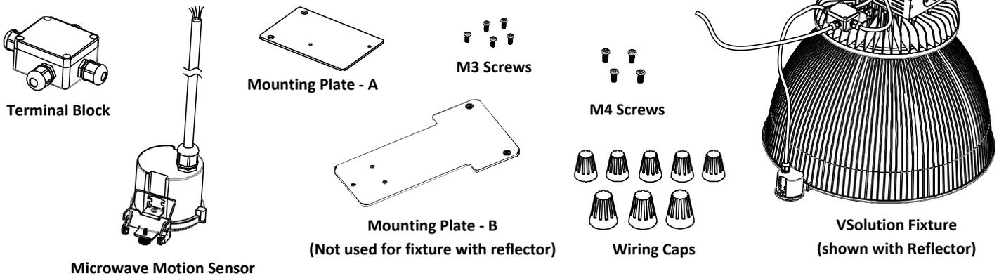
**STEP 1:** Remove terminal block cover and attach block base to mounting plate A with two M3 screws.
