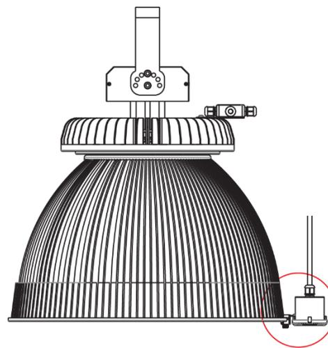
Figure 4: Tighten thumbscrew
