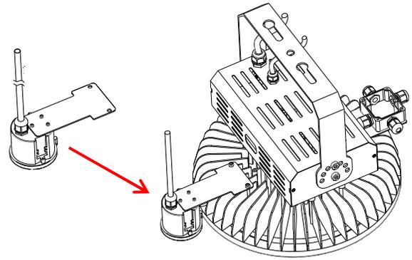
Figure 2: Attach sensor to fixture
